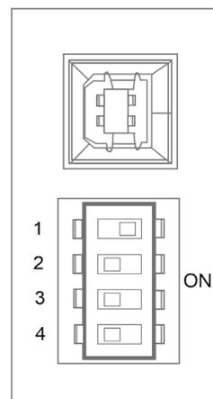
**Fig 3.3 (left)** DIP switch number 1 set to the ON position.
