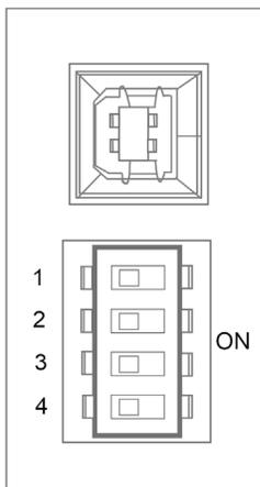
**Fig 3.2 (left)** The default setting for the DIP switches (all switches set to the OFF position).
