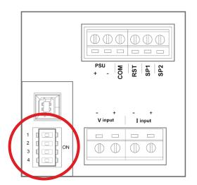
To proceed with programming, first locate the DIP switches on the back side of the Digital display. Refer to the circled area in Fig.3.1.
