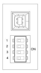
Fig 3.2 (left) The default setting for the DIP switches (all switches set to the OFF position).
